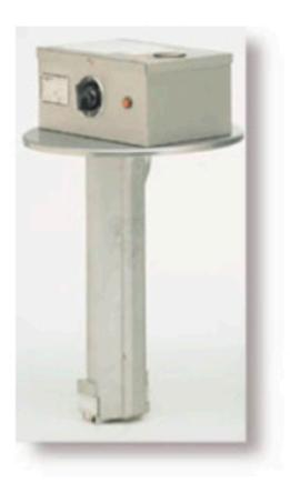
The automatic portion control pump heats, measures and delivers oil to kettle. Constructed with rugged cast aluminum heating element with 30 minute electronic timer that provides accurate portion control. For use with 50 lb. pail of oil.
